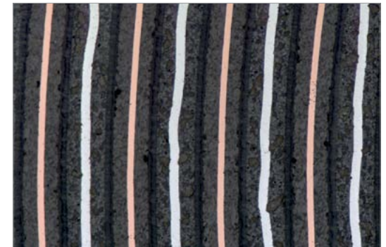
Lithium ionic accumulator, 112x, brightfield
