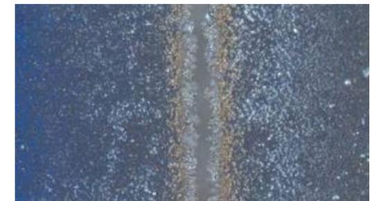
Laser edge isolation scribe: laser-textured edge isolation scribe on monocrystalline silicon solar cell;
