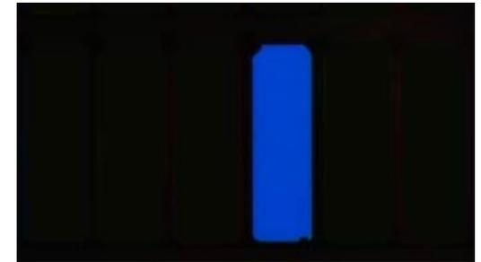
Hot stuck pixel: bright spot on black background caused by blue subpixel stuck in the "ON" state.
